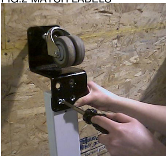
FIG.3-BOLT CASTOR TO THE BASEFRAME
