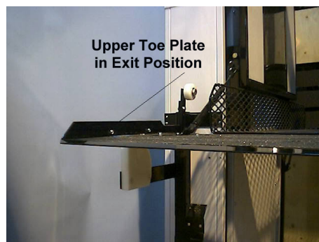
FIG.15-TOE PLATE OPENED FOR EXIT
