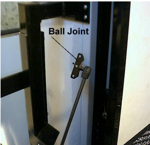
FIG.7-PRESS CYLINDER ONTO THE BALL JOINT AND MOUNT TO CARRIAGE ARM
