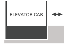
Typical Competitor 6-12 in Pit (requires extensive ground prep)
