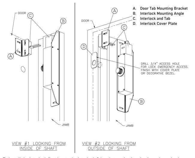
To install the interlock first locate the interlock & bracket on the door jamb as shown in view #2. With the door closed position near the top of the door jamb with the actuator tab & bracket inserted in the lock to determine the approximate position of lock and tab. Secure the interlock bracket to the jamb and the tab bracket to the door using the wood screws provided. Note that the interlock and actuator tab mounting brackets are slotted allowing for full three axis adjustment.
