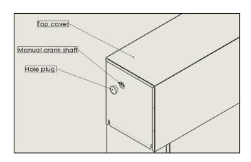
3) Push and hold the ratchet and extension into the manual crank's engaged position, as shown in the below figure, and rotate the shaft clockwise to lower the lift, and counterclockwise to raise the lift.
