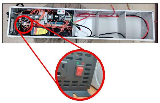
6) Wait 105 seconds, and battery power light should come on. Once you confirm that the tower is operating correctly, reinstall the front cover.
