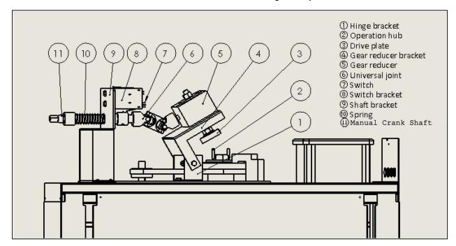
The above figure shows the normal position of the 90 Degree Manual Crank, disengaged. While the figure only shows the manual crank access on the left, the side the crank is on is specified at the time of order.
