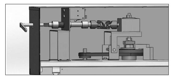
4) After the lift platform has reached the desired landing, rotate the shaft in the opposite direction approximately 5 times to relieve the load on the gearbox, and then retrieve the socket ratchet and extension to disengage the crank.
